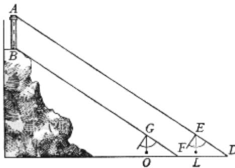
As to depths, we shall have two ways of measuring these. The first will be to measure a depth contained between two parallel lines, like the depth of a well or the [inside] height of a tower from its top. Thus, let there be the well ABCD between the parallel lines AC and DB. With the cower of the Instrument toward the eye E, sight alongside EF in such a way that the visual ray
