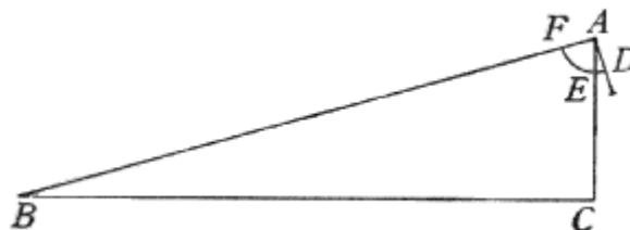
We can measure such distances in another way. Being at point A, for example, we want to find the distance to point B. Set the Instrument at right angles, one leg being pointed toward B. and sight along the other leg toward point C. Measure 100 paces (or other units) in the direction AC and leave a staff driven at
