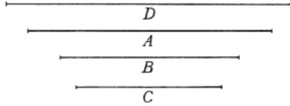
To do this, take with a compass line A, which is applied to some point on the Stereometric Lines; let this be for example to points 30-30. Not moving the Instrument, consider the number B fits; and finding it to fit, for example, at 12, add that at which line number to the number 30 already mentioned, getting 42, to be held in mind.
