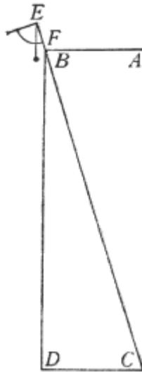
passes through points B and C, noting the number cut by the thread, which for example let be 5. Then see how many times this number goes into 100, and that many times will the breadth BA [which can be measured] be contained in the depth BD.
